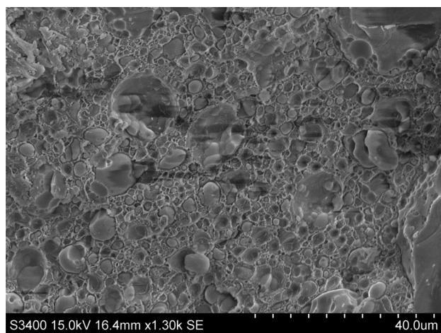
Figure 3. Characteristic cryoSEM image of poly(silicone)MIPEs produced from an emulsion template with 50% internal phase volume ratio containing 30 g L -1 \text{NaHCO}_3 solution, agitated for 45 s.
