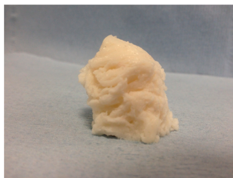
Figure 6. Damaged polyMIPE produced by curing an MIPE template with 70% internal phase (sample 17) after removal from the mold. Compare this polyMIPE to the polyMIPE monoliths produced by curing MIPEs with an internal phase of 50 and 60% (Figure 3).
